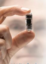
The CapsoCam Plus capsule is approximately the size of a large multi-vitamin and can be swallowed with a few sips of water.
